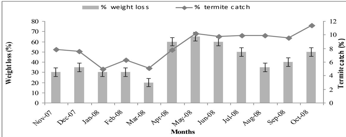
**Fig 1.** Seasonal wood degradation and total termite catch in different months (2007-08) in Nallal (Bar indicates standard error of the mean)
