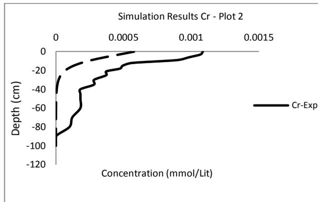
Fig 1. Experimental and simulation results of Cr concentration after 150 days plot 2
