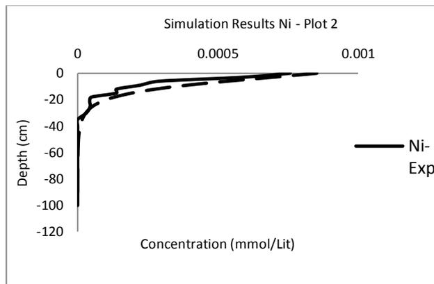
Fig 2. Experimental and measured results of Ni concentration after 150 days plot 2
