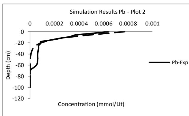
Fig 3. Experimental and simulation results of Pb concentration after 150 days plot 3
